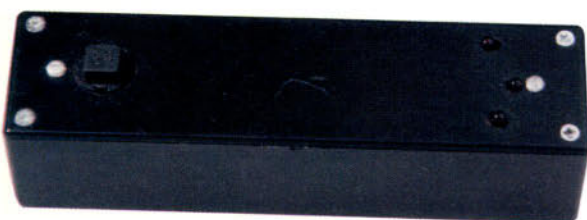
Photo 1: The prototype infra-red transmitter. Note the spacing of the three diodes (see text).
