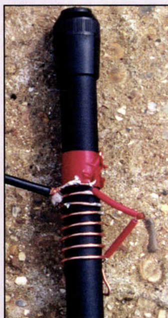
Fig. 2: The coil and fixed capacitor resonate at about 50.125MHz. The capacitor has its 'legs' insulated.
