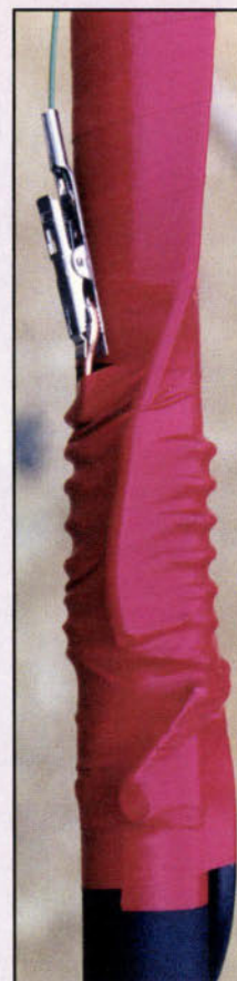
Fig. 6: The final loading coil wrapped up in electrician's insulating tape. The coaxial capacitor runs up the pole under the tape.
