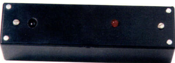
Photo 2: The remote receiver. The inset diode is the infra-red detector and the 'proud' diode on the right is the operating indicator (see text).
